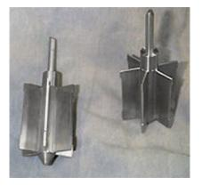
**Solution:** Our customer chose electropolishing to provide a clean and passive surface. Electropolishing removed the imbedded oxides from machining and polishing compounds with a controlled amount of material removal. After electropolishing the part is clean, passive in tolerance and ready for assembly.
