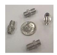
**Note to engineer:** Parts fabricated oversize or that have grown in size due to heat treating generally respond well to salvaging via electropolishing. Bear in mind that sizing applications requiring lower ranges of stock removal (.002" or less) IN GENERAL respond better. In addition, we can mask or favor certain areas of larger or more complex parts. If you have an oversize part that may be a candidate for salvaging, please send samples or provide a blueprint for specific recommendations.
